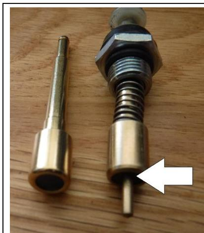
The effect that high ethanol levels in modern fuels have on the rubber components in carburetors is well documented. If the rubber in the end of the choke plunger (arrow on the right) goes hard and fails to seal the choke, allowing air to bleed past, then it is effectively running with choke on all of the time.
