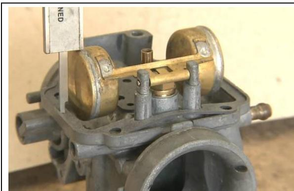
In practice, you can get a reasonably good check by allowing the floats to rest held down by their own weight (gravity), when upside down for measuring.
