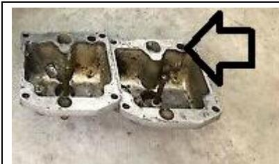
The choke mechanism draws fuel from the float bowl via a hole as shown here.
